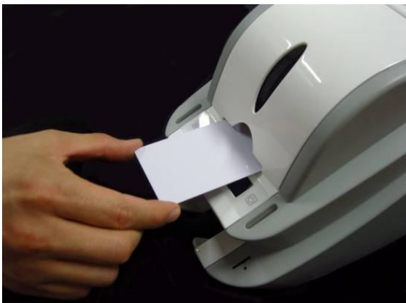
Pic.27 Loading the cards 3
